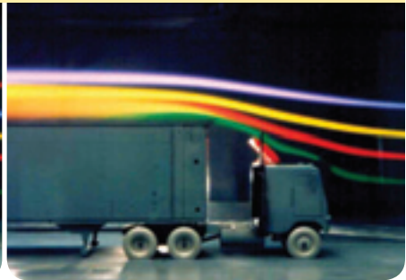
Figure 2: Comparing air movement with and without a cab roof deflector 1
