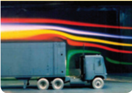
Figure 2: Comparing air movement with and without a cab roof deflector 1
